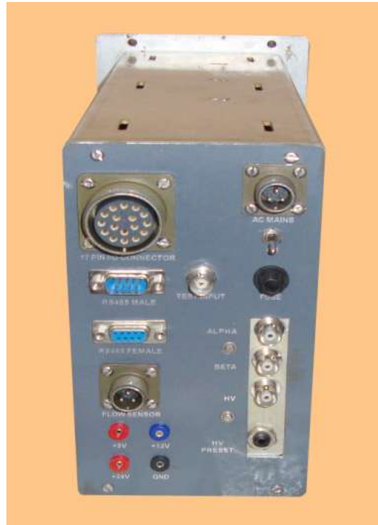
Fig (3) ELECTRONIC UNIT REAR VIEW
