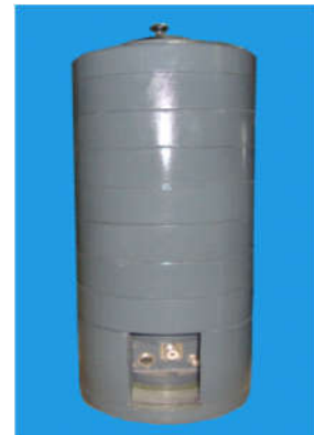
3 - Inch detector (10 lead assembly parts)
