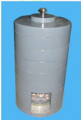
1- Inch detector (8 lead assembling parts)
