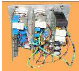
Fig : Amp-SCA module electric circuit PCB arrangement
