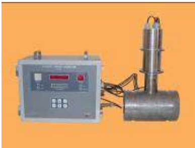
Fig : On-line gamma monitor unit with S.S. On-line gamma probe fixed into a sample pipe-line flange with lead shielding arrangement including clamps.
