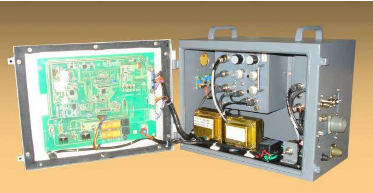
Fig : Inside view of On-line gamma monitor showing electronic arrangement
