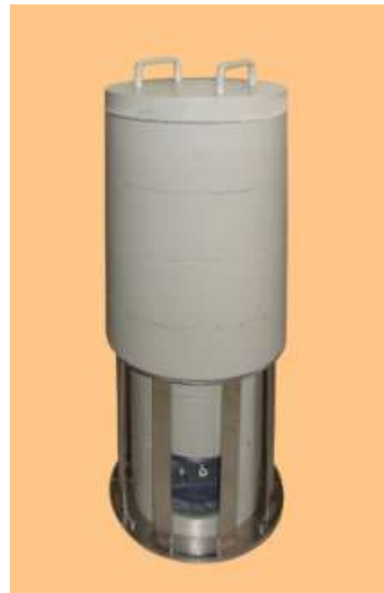
3"x3" NaI detector covered with Lead shielding arrangement
